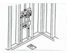
3. Remove the tub and install the drain, predrill holes on the tiling flange at the marked location of the studs.
