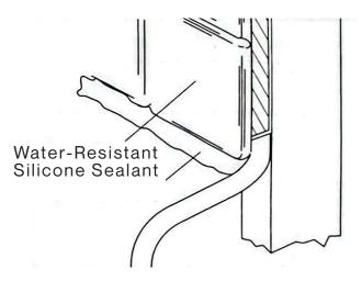
8. Install water resistant gypsum board and finish surface material (tile, stone) and seal all edges with silicone caulking to prevent water damage.
