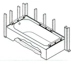
5. Move tub into place, make sure the tub is level and plumb. Adjust feet or shim as necessary. The tubs weight should be supported on the feet. Make sure that the mortar bed is in contact with the entire tub basin.
