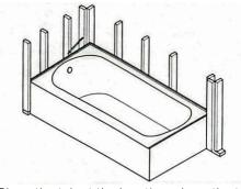
2. Place the tub at the location where the tub will be installed, level tub on all sides and mark the location of the drain and the wall studs on the tiling flange.
