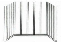
1. Prepare area by framing the area where the tub will be installed.
