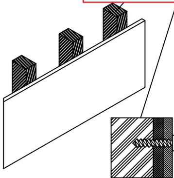
**STUDS:** Secure to wall with ST4.2\*70mm screws at stud location. Locate at least 2 wall studs
