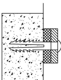
**CONCRETE:** Drill 1/4" holes, insert #10 wall anchors and secure to wall with #10 x3" screws.
