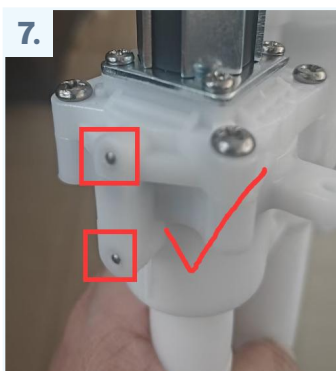
Retighten the screws of the solenoid valve in the correct direction.
