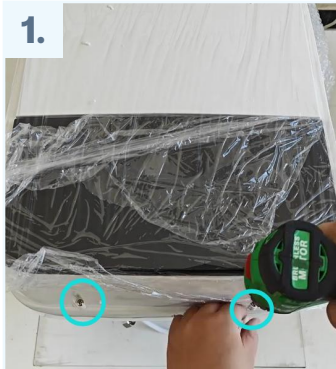
Loosen the cover screws.
